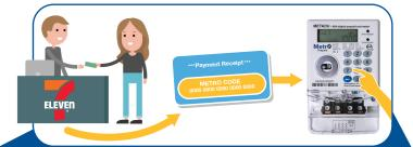
When a Metro Code is purchased, the code is printed on a cash slip, e-mailed or sent by text. This Metro Code is then keyed into the sub meter and the meter is recharged.
